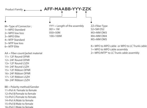
In the above part No. scheme substitute the given code No, or letter to arrive at the cable assembly ordering part number
