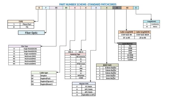
In the above part No. scheme substitute the given code No, or letter to arrive at the cable assembly ordering part number
