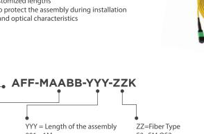
M=Type of Connector; 1= MPO Standard 2= MPO low loss 3= MPO Flite 4= MTP Standard 5= MTP low loss
